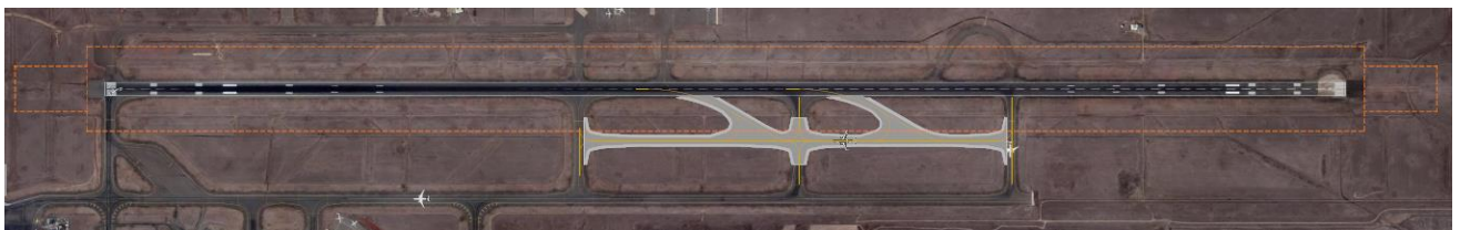
Figure 160: Phase 0 of the proposed runway and taxiway system expansion (RETs and parallel taxiway, 2026)
