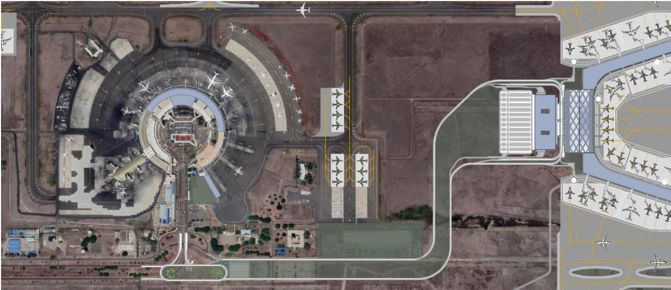
Figure 188: Rerouting of existing roads to access the new Terminal and associated parking and curbside
