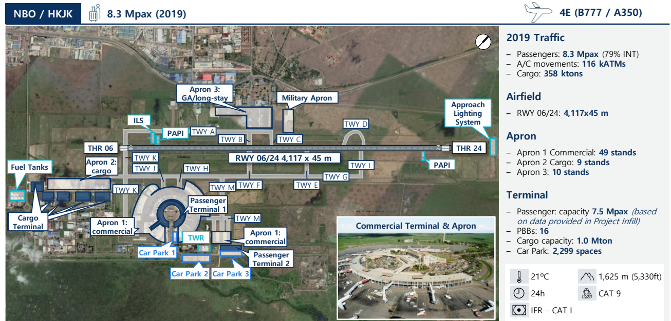
Figure 124: Overview of Jomo Kenyatta International Airport (Source: Google Earth, AIP, KAA, CAPA)
